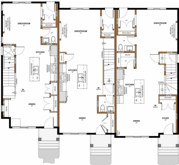
FIRST FLOOR PLAN A: 713 sq ft FIRST FLOOR PLAN A: 721 sq ft FIRST FLOOR PLAN A: 814 sq ft
